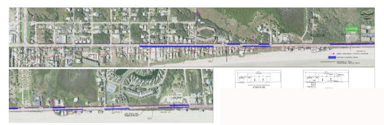
The above rendering represents the proposed 8- foot trail and drainage improvements to Coastal Highway from the State Road A1A intersection to 24th Street to reduce roadway flooding.
