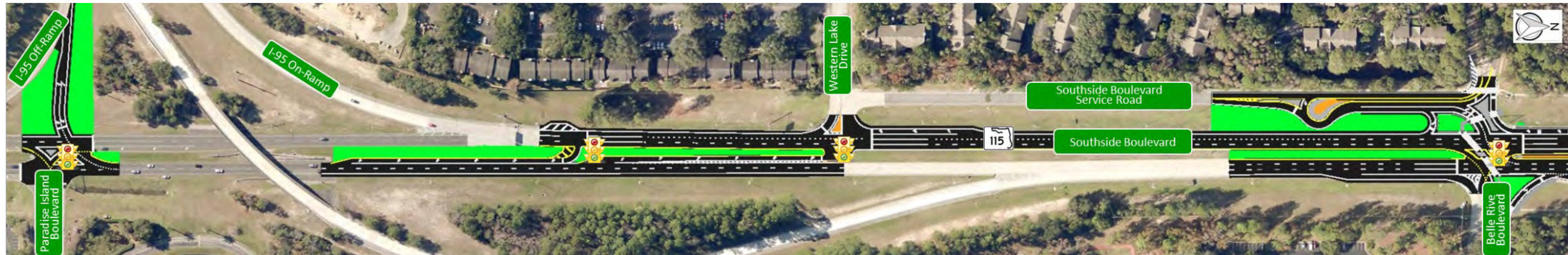
The Paradise Island Boulevard and Southside Boulevard intersection will be modified to accommodate the I-95 northbound off-ramp left turn movement. The Belle Rive Boulevard and Southside Boulevard intersection will be modified as shown.
