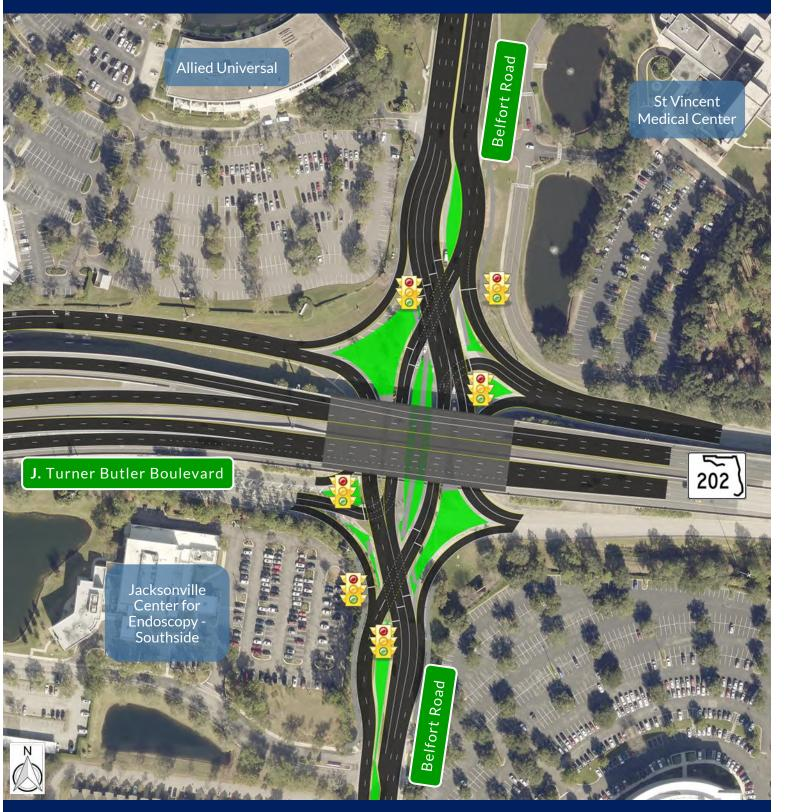
The J Turner Butler Boulevard at Belfort Road interchange will be converted to a Diverging Diamond Interchange as shown. Belfort Road will be widened to accommodate two through lanes and two left turn lanes in both directions. The through movement will be eliminated at the exit ramps, and an additional right turn lane will be provided for the westbound exit ramp.
