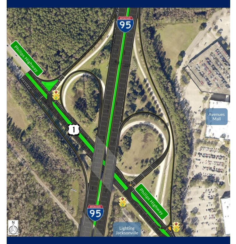
The I-95 at Philips Highway interchange will be modified as shown. The existing free-flow I-95 northbound exit ramp to Philips Highway northbound right turn movement will be signalized, and a lane will be added to the I-95 southbound exit ramp.
