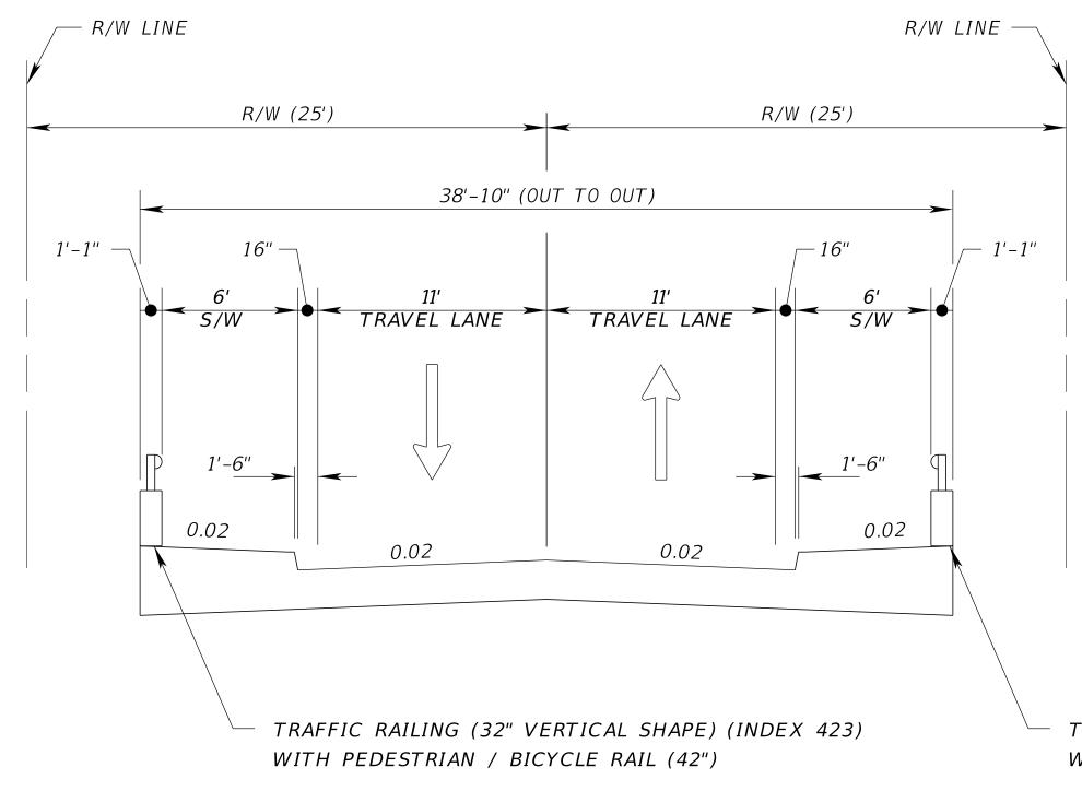
TRAFFIC RAILING (32" VERTICAL SHAPE) (INDEX 423) WITH PEDESTRIAN / BICYCLE RAIL (42")
