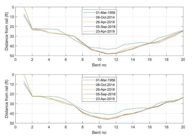
FIGURE 6-2: SCOUR – LEFT AND RIGHT PROFILES
