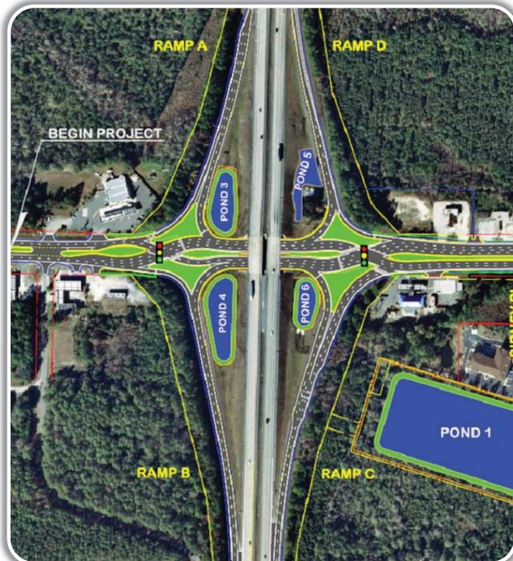
A diverging diamond interchange (DDI) is a type of interchange where the two directions of traffic below I-95 briefly drive on the opposite side of the road. This will be a significant improvement in safety, since long left turns crossing traffic lanes to enter or exit the Interstate will be eliminated.
