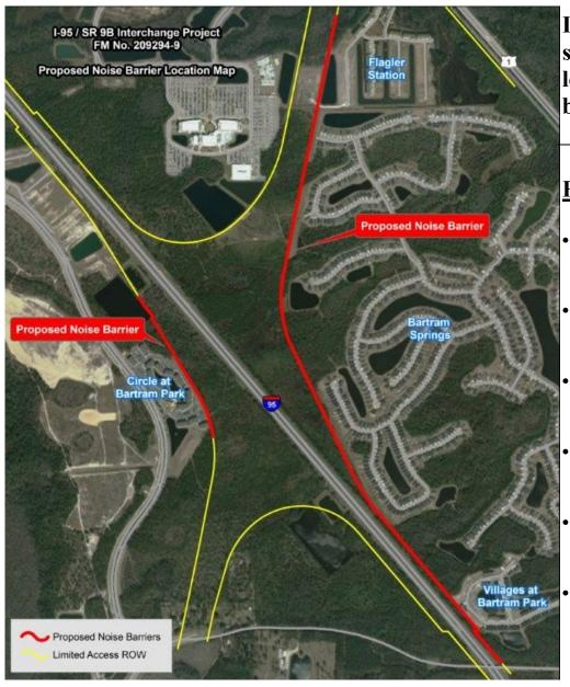
Image at the left shows the proposed location of noise barrier walls.
